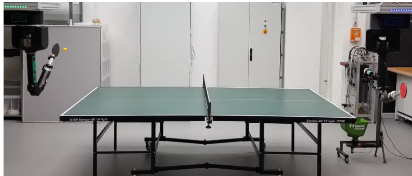
Figure 1.12: In the past, we have studied a single robot playing table tennis against a human or ball gun. In 2018, we migrated to a new lab and a setup with two robots. We aim to enable the unique high-speed Barrett WAM robot arms PING and PONG to jointly play table tennis in a collaborative game using methods from robotic skill learning.
